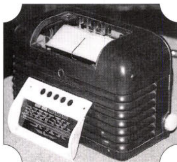
Fig. 7: Because of its push-button tuning facility, the Bush DAC10 was useful for blind listeners.
