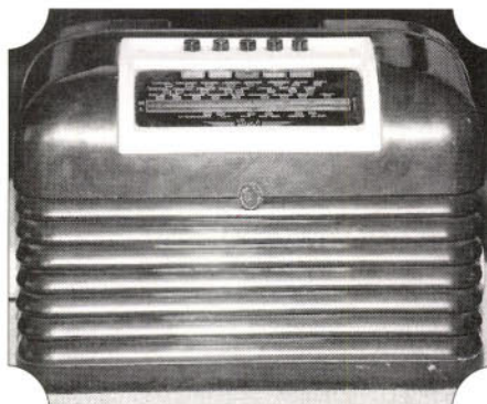
Fig. 2: The Bush DAC10 used miniature glass-based valves (see text).
